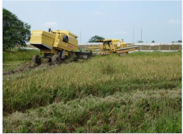
Heavy machineries sink in submerged soil
