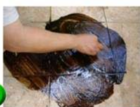
5 Cleaner is mixed thoroughly with dirty oil using brushing application.
